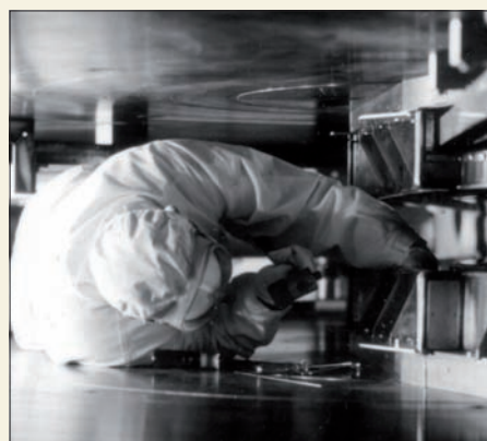
Because of the radioactivity inside the cyclotron vacuum tank, work there has to be carried out quickly and accurately. This is not helped by the narrowness of the gap between the two magnet poles, as this picture shows.
