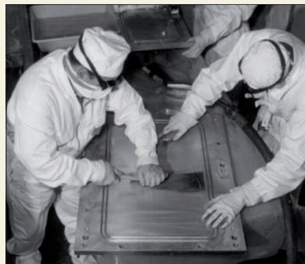
This photograph shows some cover plates from the vacuum chamber of the SC being cleaned inside a concrete enclosure set up in the “proton” experimental room. As the plates were radioactive, the cleaners had to wear overalls, masks, goggles and gloves, and their stay inside the enclosure was carefully controlled.
