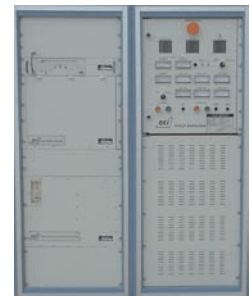
25KW, 18-32MHz, CW, Water Cooled, RF Amplifier
