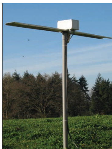
Top: A view of the antennas of the Decametric Array that CODALEMA uses at the Nançay Radio Observatory. Above: One of the 16 active wide-bandwidth dipole antennas with its application-specific integrated circuit layout (right).
